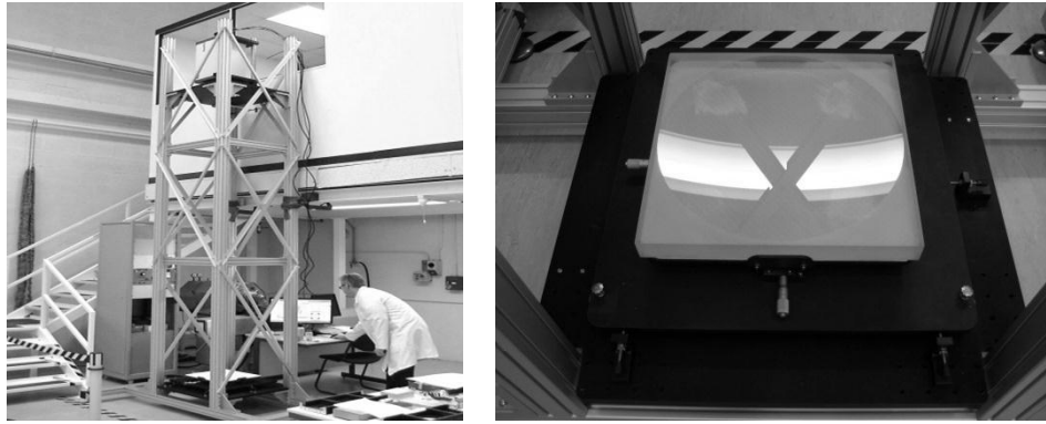
Figure 3. Optical test tower overview (left), Optical test tower lower platen (tip/tilt/power correction) (right)
