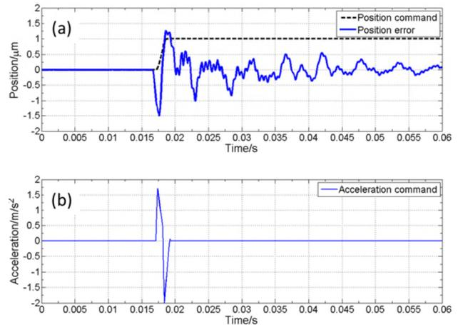
Figure 3. Position step command and position error (a), acceleration command (b).
