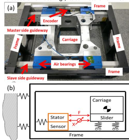
Figure 1. Linear motion module (a), motion system 2D model with (b).
