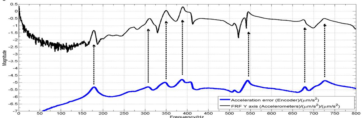
Figure 4. Comparison between acceleration error FFT and acceleration FRF in the motion direction.
