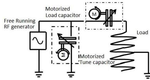
Figure 3. Motorized fixed match RF network.
