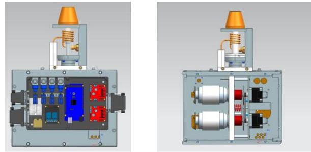
Figure 4. Electrical components (left), Mechanical components (right).
