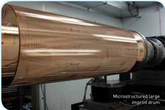
Laser machined glassy carbon imprint tool
