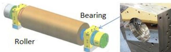
Figure 1. Diamond turned rollers and Hydrostatic bearings & housing.
