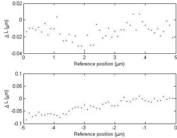
Figure 5. The difference between the displacement measured by a chromatic probe and the reference position as measured by a precision motion system ( $\Delta L$ ), moving from 10  $\mu\text{m}$  to 15  $\mu\text{m}$  (top) and 290  $\mu\text{m}$  to 285  $\mu\text{m}$  (bottom) as measured by the chromatic probe.
