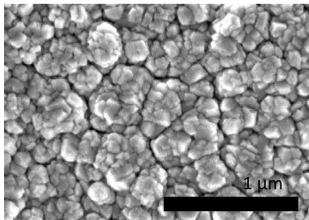
**Figure 3.** High resolution SEM images of W deposited on Si showing lateral grain dimension of 100-300 nm.
