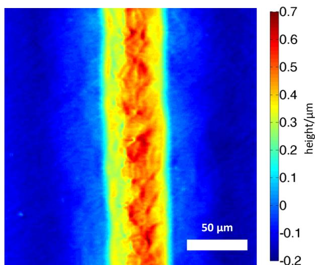
**Figure 2.** Deposition height profile measured using WLI and done by scanning the laser at 2.4 W in the presence of the precursor at a speed of 0.18 mm/s on SS.
