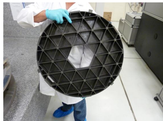
FIGURE 7. Light weight silicon carbide mirror substrate produced by Boostec of France
