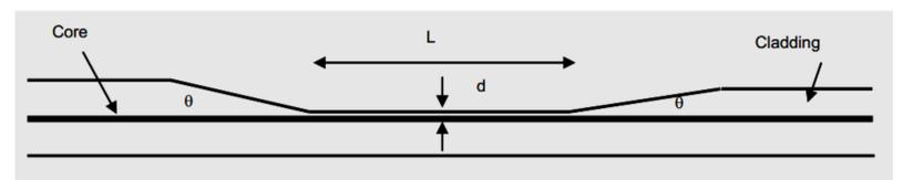
The sensing behaviour is highly dependent on the depth the cladding is polished to. The fibres currently used have large tolerance values on this depth.
