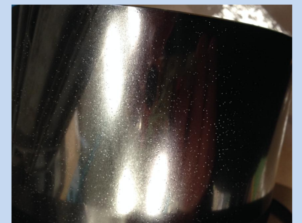
Visible pitting on diamond turned spindle sample with 75μm electroless nickel coating, Image: Poeton
