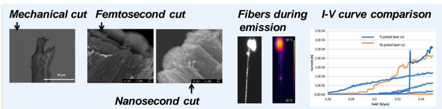
Comparative emission trials between straight and triangular geometries on films has been carried out. Stacks of triangular films gave the highest emission, up to 7.6mA, with temperatures at the tip being below 840° C.
