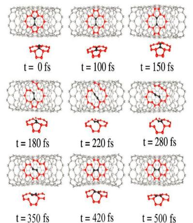
Rotated dimer (black) after interaction with a Gaussian shaped laser pulse (50fs). Taken from Valencia 2006
