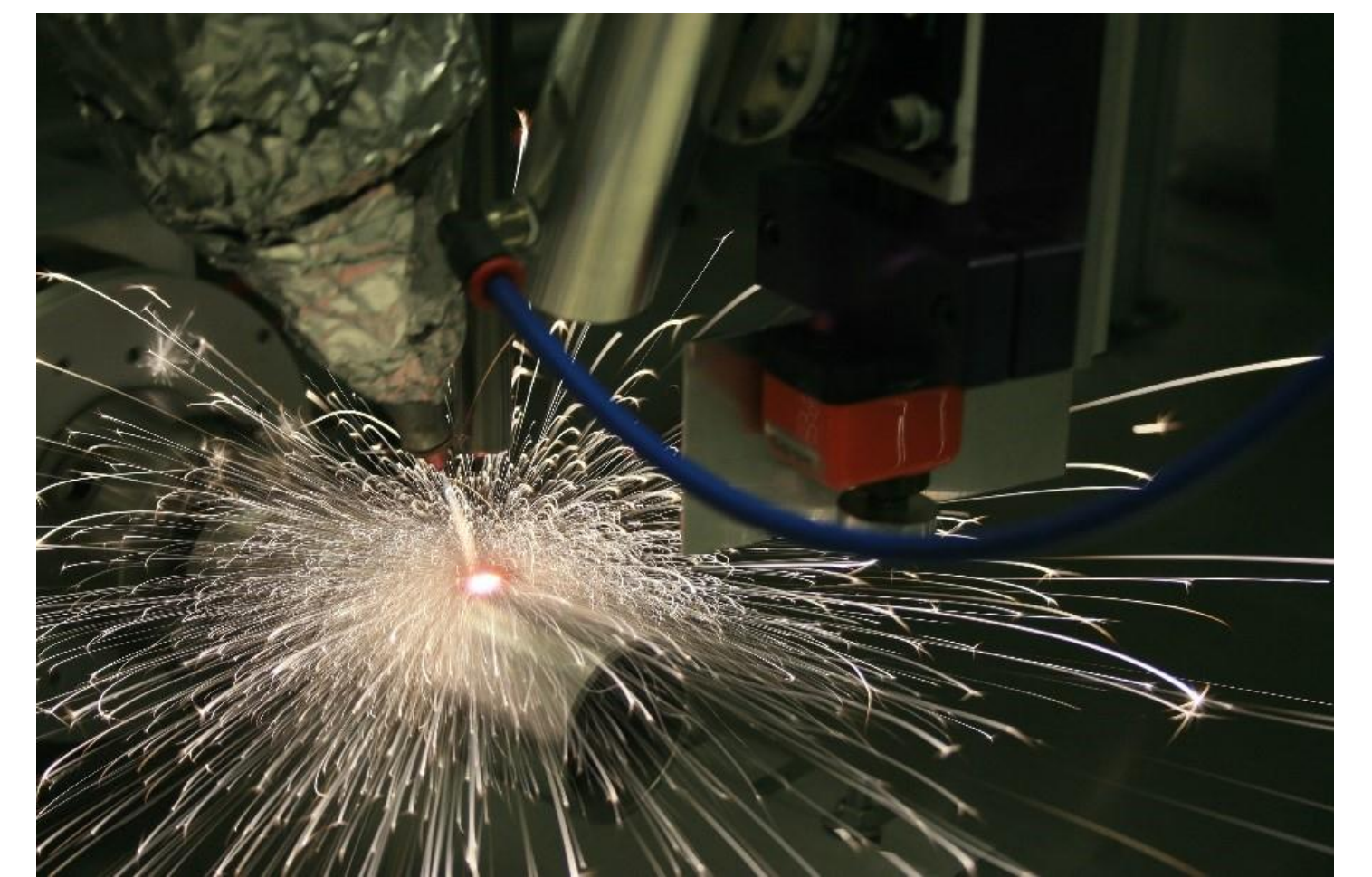
Figure 2: The existing SLD process in action.
