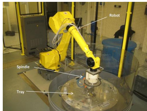
Figure 5: Industrial robot based polishing system
